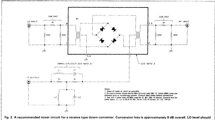
be between 5 and 15 milliwatts. If a 28 MHz IF is not used, the diplexer must be modified as described in text. See text for other recommended dBm's.
